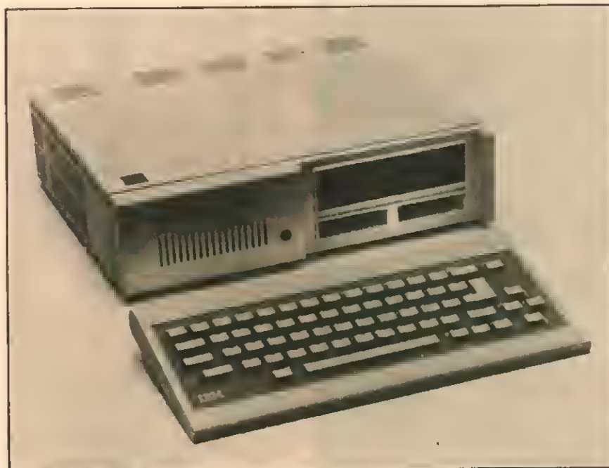
The PCjr: keyboard and disk-drive-equipped system unit.
